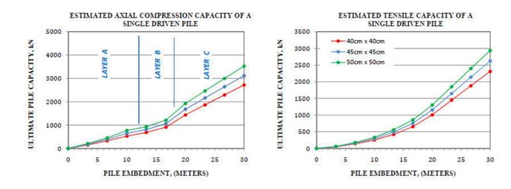
Figure 7-2. Estimated ultimate capacity of single-stick driven piles
