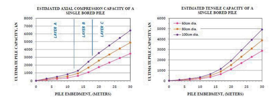
Figure 7-2. Estimated ultimate capacity of a single bored pile
