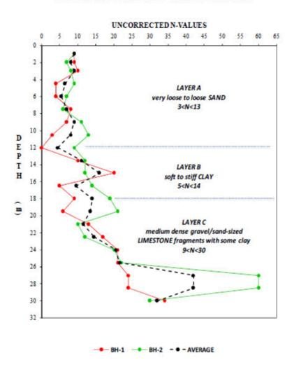
Figure 6-1. Plot of uncorrected N-values vs. depth
